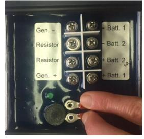
6. Place the screws into the holes so that the two metal disks around each screw lie on top of each prong, and use a screwdriver to tighten until the prongs of the remote temperature probe are firmly secured to the surface of the charge controller.
