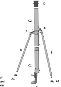
Mast components made of polished 316L Stainless Steel. 16ga Wall thickness 2.25 OD See Pg 27 of the Superwind Manual for installation instructions for the Superwind.
